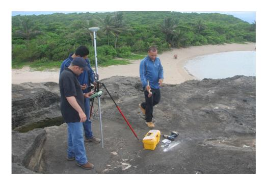
Figure 31: Employees of Vernix Engineering installing and measuring Punta Manatí benchmark.
