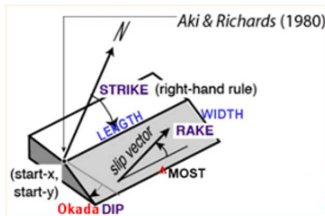
Figure 8 – Fault plane showing locations used to locate it. The red triangle at the middle of the bottom edge is the location expected by MOST.
